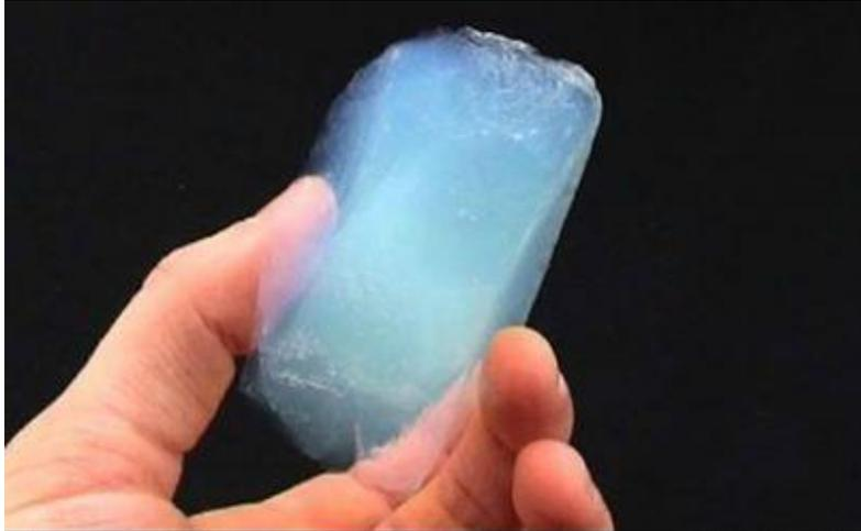
**Aerogel, also known as frozen smoke, is the world's lowest density solid, clocking in at 96% air. If you hold a small piece in your hand, it's practically impossible to either see or feel, but if you poke it, it's like styrofoam. It supports up to 4,000 times its own weight and can withstand a direct blast from two pounds of dynamite. It's also the best insulator in existence.**
